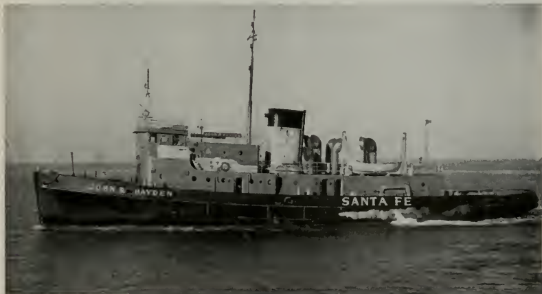
View of the John R. Hayden, 149 foot, 581-ton, 1200 hp, all steel tug of the Santa Fe Railway marine fleet, in operation in San Francisco Bay.
